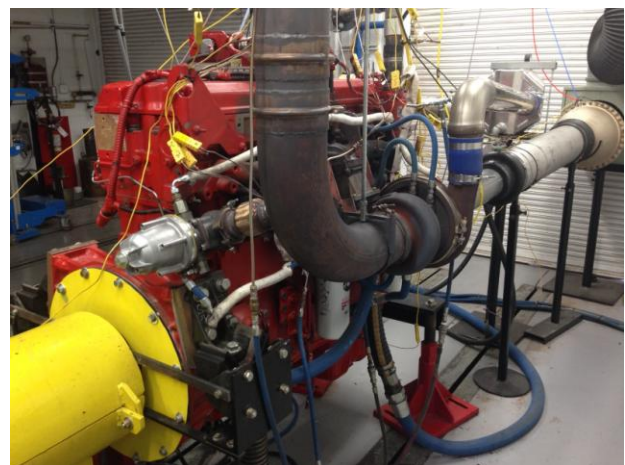
Figure 2: 850 HP Cummins ISX15 test engine.
